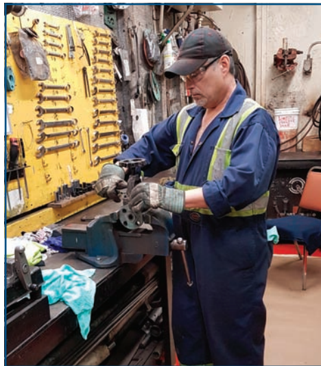
Engine Room Attendant Carson Jacque carries out repair work on a valve.
