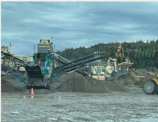
Vale added two new Metso crushers and a Chieftain screener to handle the increased demand for crushed rock since the underground project began.
