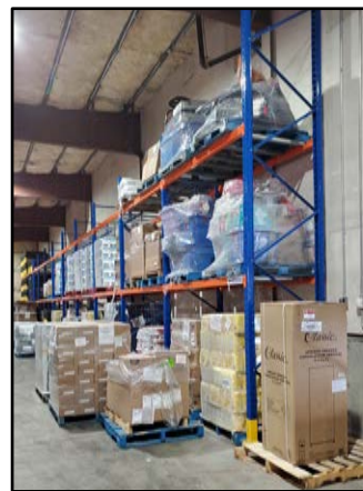
Investments at the freight terminal in Goose Bay helped improve the safe storage and movement of freight. Above left, steel racking was installed to allow for vertical stacking of freight which also increased capacity. Above right, new electric forklifts improved productivity around freight operations and contributed to the successful 2020 season. (Gary Latimer photos)
